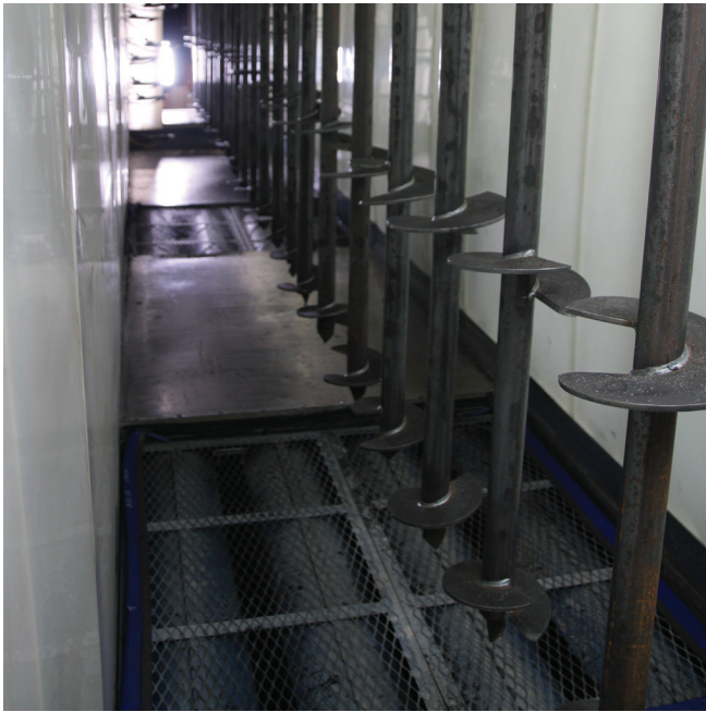
FIGURE 6-6 : Helical Lead Sections Hung From Conveyor System
