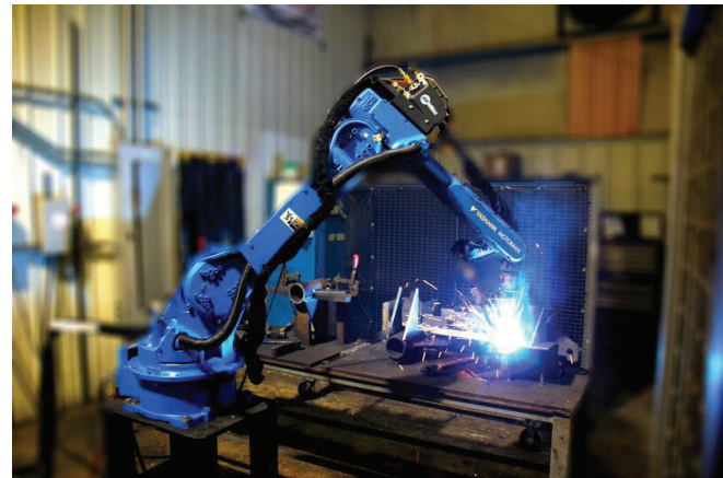
FIGURE 1-4 : Ram Jack Robotic Welder
