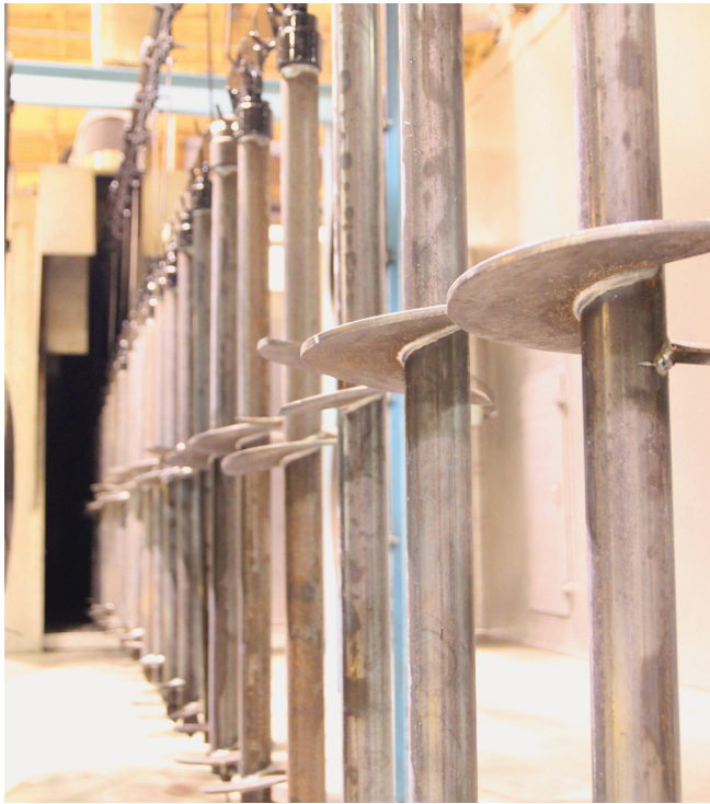
FIGURE 6-7 : Helical Lead Sections Leaving Shot Blast Cabinet
