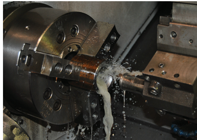
FIGURE 1-7 : Machining Threaded Connections
