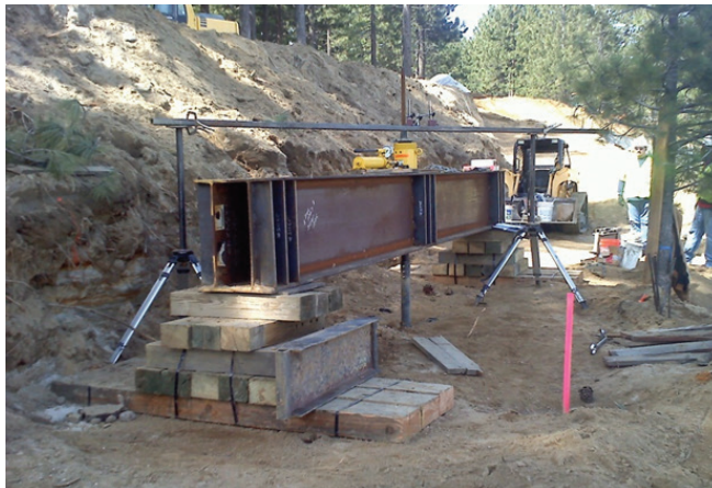
FIGURE 3-17 : Performance Tension Load Test Setup on Helical Anchor
